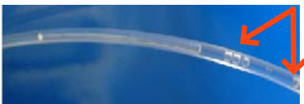
Figure 6 HPFA+ Tubing Showing Broken Air Gap
