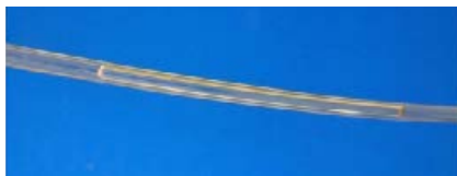
Figure 5 Radel R Tubing Showing Intact Air Gap
